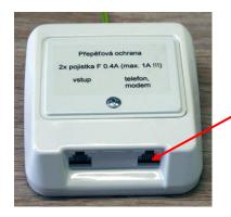
The socket is larger than the cable connector. However, the socket is adaptive, so a cable with an connector RJ 11 must be used.
