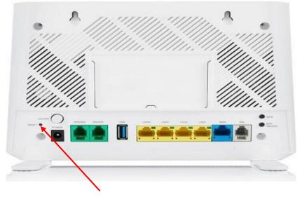
Press the reset button with a toothpick, pin, or open clip for at least 15 seconds.
