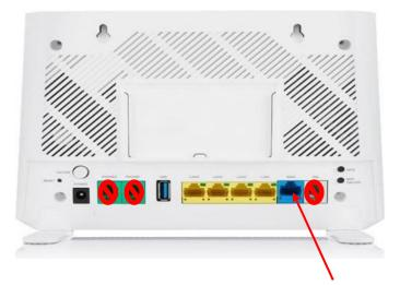
We plug the cable with the RJ 45 end into the WAN port.
